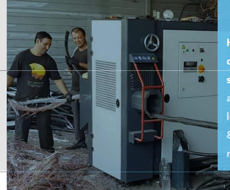
Heavy duty cable stripper strips steel (tape) armoured cable, lead covered cable & thick nylon ridged cables
